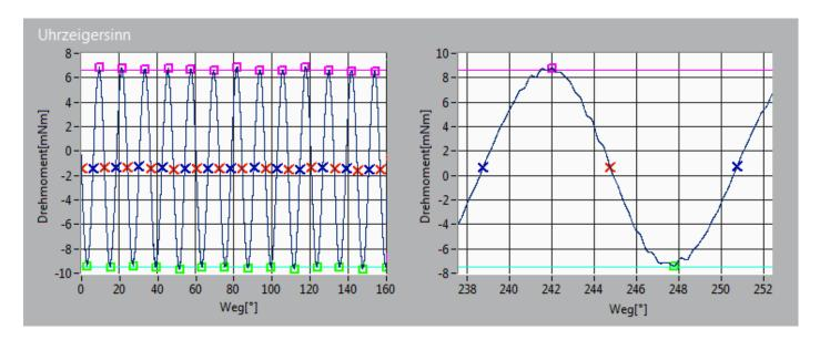
The DTN 38 can be used to verify the suitability of the rotary haptic module DHM as a measuring system in accordance with the guidelines on "Capability certification of measuring systems". (tolerance range  $T \ge \pm 5.00$  mNm; cgk value  $\ge 2.00$ )
