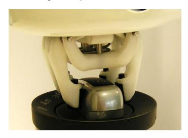
A special, in the gripper integrated mechanism uniformly distribute the locking force to all four fingers. The fingers adapt oneself by closing at the outline of the switch and ensure a stiff touch of each finger to the surface of the switch.
