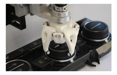
The rotary haptic grippers in the DHG3 series have been specially developed for use in rotary haptic measuring systems. They have been optimized with regard to the mass moment of inertia and torsion resistance, while their high reliability and torsion resistance have been demonstrated in many applications.
